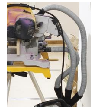
Three point dust extraction
