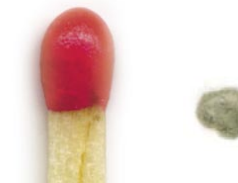
An amount of RCS dust smaller than a match head inhaled over a full shift can put your health at significant risk
