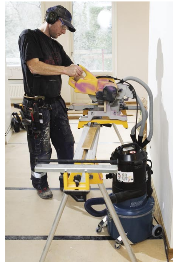
Three point dust extraction
